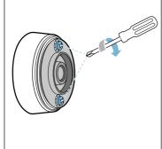
**4.** Reattach the silicone cover to the lower section of the temperature sensor housing.
