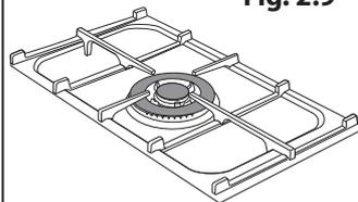
**Note:** The use of aluminium pans may cause metallic marking of the pan supports. This does not affect the durability of the enamel and may be cleaned off with an appropriate metal cleaner.
