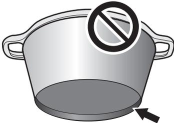
The minimum recommended pan diameter is 120 mm. The maximum allowable pan base diameter is 260 mm. For a pan diameter of 120 mm, or less, use the additional pan support trivet supplied (Fig. 2.8).
