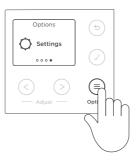
Press OPTIONS  $\equiv$ , scroll to SETTINGS using the ADJUST  $\langle \rangle$  buttons, press  $\sqrt{}$  to confirm.
