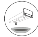
2. Dump the condensate water and reinstall the water box in place.
