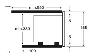
NB. For under bench installation please allow 100mm clearance from cabinetry to the floor
