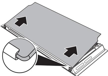
4. Remove the intermediate glass unit by lifting it upwards.
