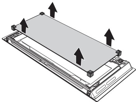
5. Clean the external glass pane and the panes removed previously. Use absorbent kitchen roll. In case of stubborn dirt, wash with a damp sponge and neutral detergent.
