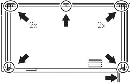
**Position of the screws and the power cable
